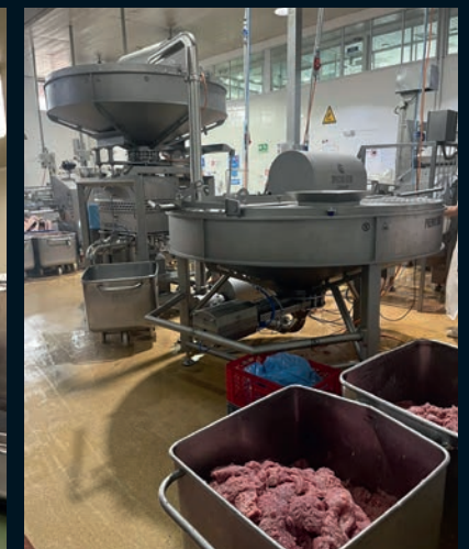
Line configuration: TT BASTARD 160 + PREMIX 1000 WITH PRE-PUMP + PREMIX 1000
