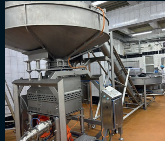
Line configuration: TT BASTARD 160 + PREMIX 1000 WITH SCREW CONVEYOR
