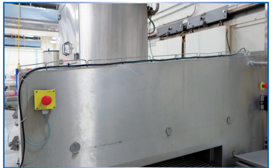
HYGIENICALLY DESIGNED SLOPED SURFACES FOR WATER RUNOFF
