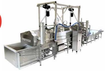
Our CK1500 cooker enables you to cook open unpacked food continuously. It has a modular design - making it ideal for different outputs. The CK1500 is available as a free-standing unit or to be integrated into an entire cooking line.
