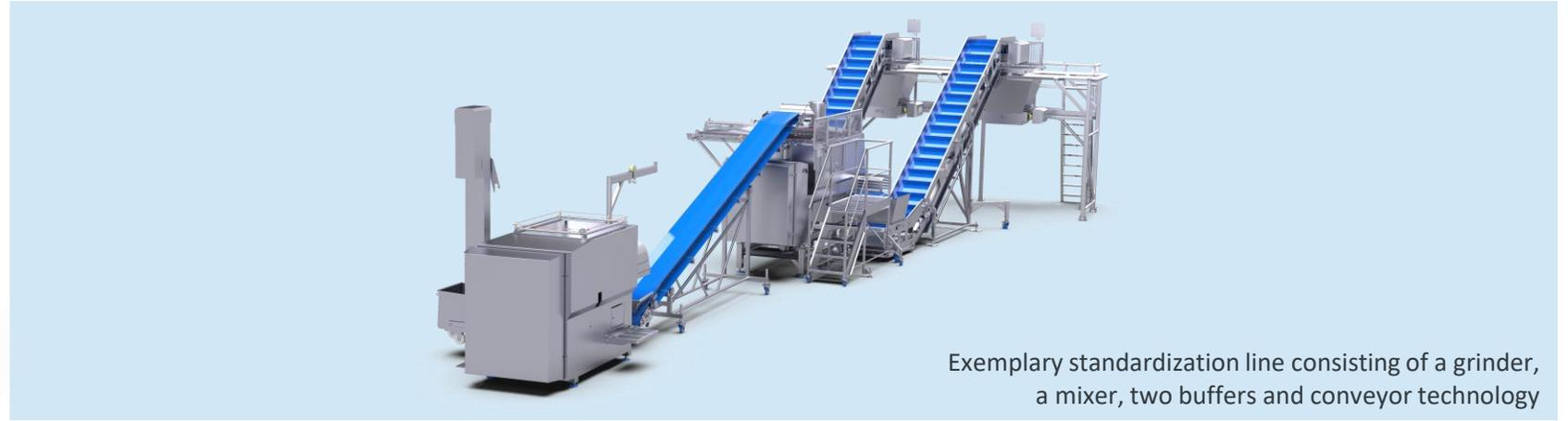
Exemplary standardization line consisting of a grinder, a mixer, two buffers and conveyor technology
