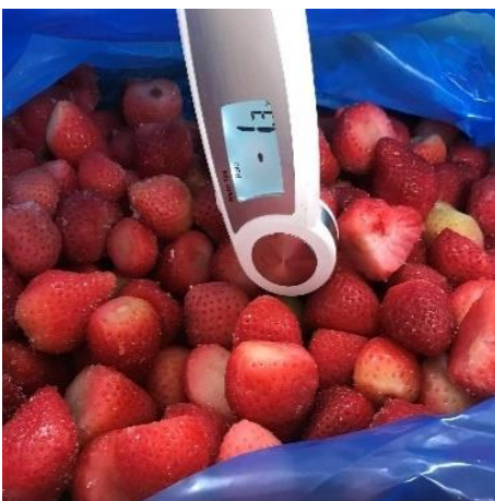
Strawberries 10 kg bags 950 kg/h from -18^{\circ}\text{C} to -3^{\circ}\text{C}/-1^{\circ}\text{C}
