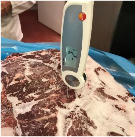
Beef 25% fat, 25 kg 1500 kg/h from -18^{\circ}\text{C} to -4^{\circ}\text{C}/-2^{\circ}\text{C}
