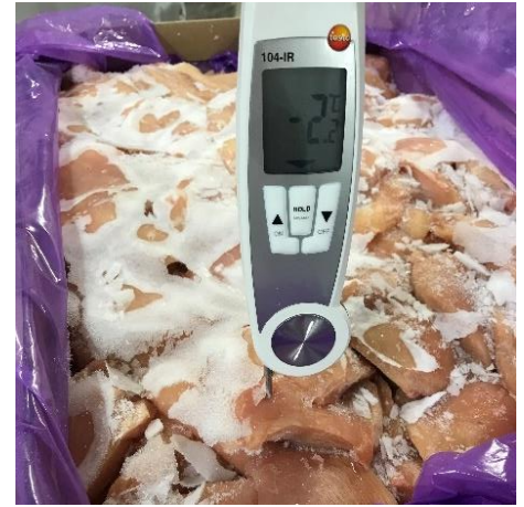
Chicken breasts 15 kg 950 kg/h from -18^{\circ}\text{C} to -4^{\circ}\text{C}/-2^{\circ}\text{C}
