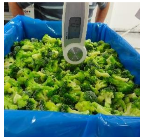
Broccolis 20 kg bags 900 kg/h from -18^{\circ}\text{C} to -3^{\circ}\text{C}/-1^{\circ}\text{C}
