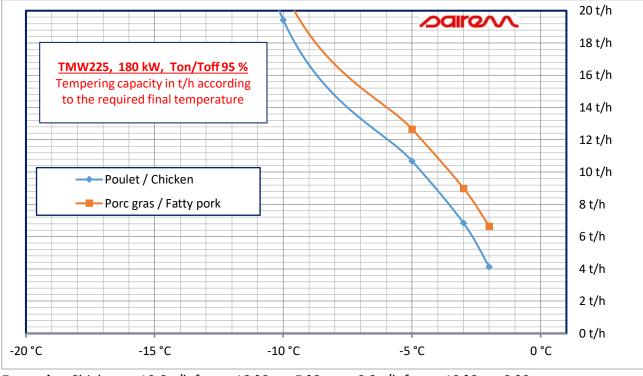
**Example:** Chicken  $\simeq 10.8$  t/h from -18 °C to -5 °C or  $\simeq 6.8$  t/h from -18 °C to -3 °C. **Example:** Fatty pork  $\simeq 12.7$  t/h from -18 °C to -5 °C or  $\simeq 9$  t/h from -18 °C to -3 °C.
