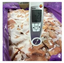
Chicken breasts 15 kg 5000 kg/h from -18°C to -4°C/-2°C Block size: 600 x 400 x 260 mm
