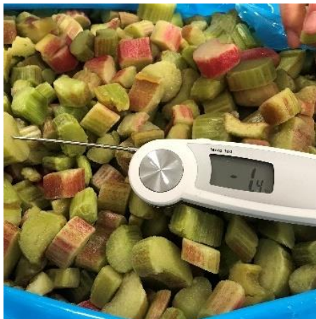
Rhubarb 100 kg bags (10 x 10 kg) 2500 kg/h from -18 °C to -3 °C/-1 °C
