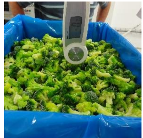
Broccolis 100 kg bags (10 x 10 kg) 3400 kg/h from -18 °C to -3 °C/-1 °C
