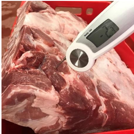
Pork shoulder 10 to 15 % fat, 25 kg 4000 kg/h from -18 °C to -3 °C / -1 °C Block size: 600 x 400 x 260 mm
