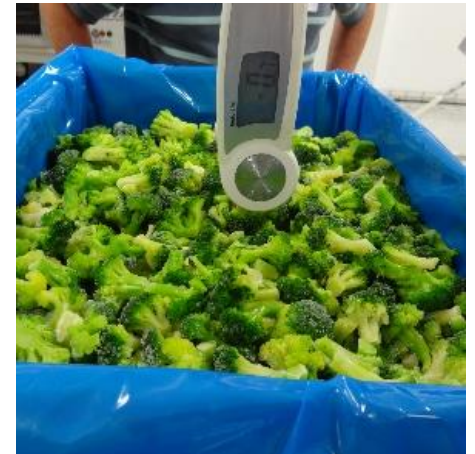
Broccolis 20 kg (1 x 20 kg) Capacity: ≈ 160 kg/h from - 18 °C to - 3 °C/- 1 °C
