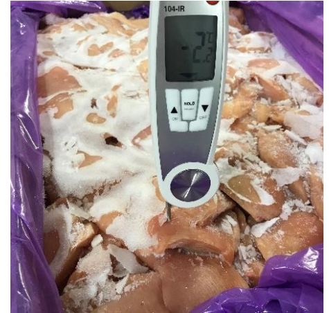
Chicken breasts, 15kg (1 x 15kg) Capacity: ≈ 140kg/h from -18°C to -4°C/-2°C
