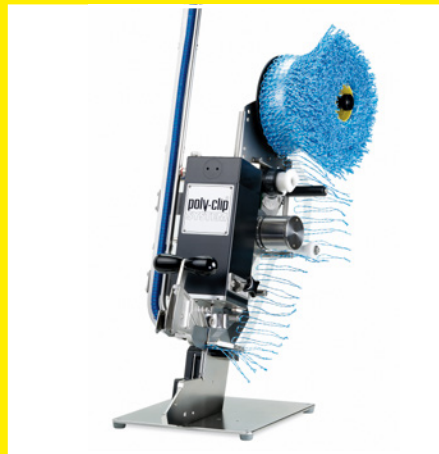
Version with pneumatic cutter and GSE (automatic looper)
