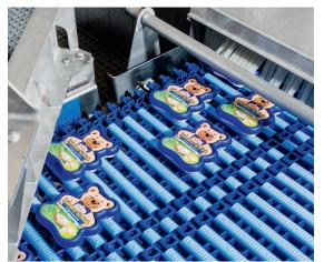
A belt with a special rubber coating as well as the DirectDrive system ensure the conveyor will run smoothly and keep the products in their positions.
